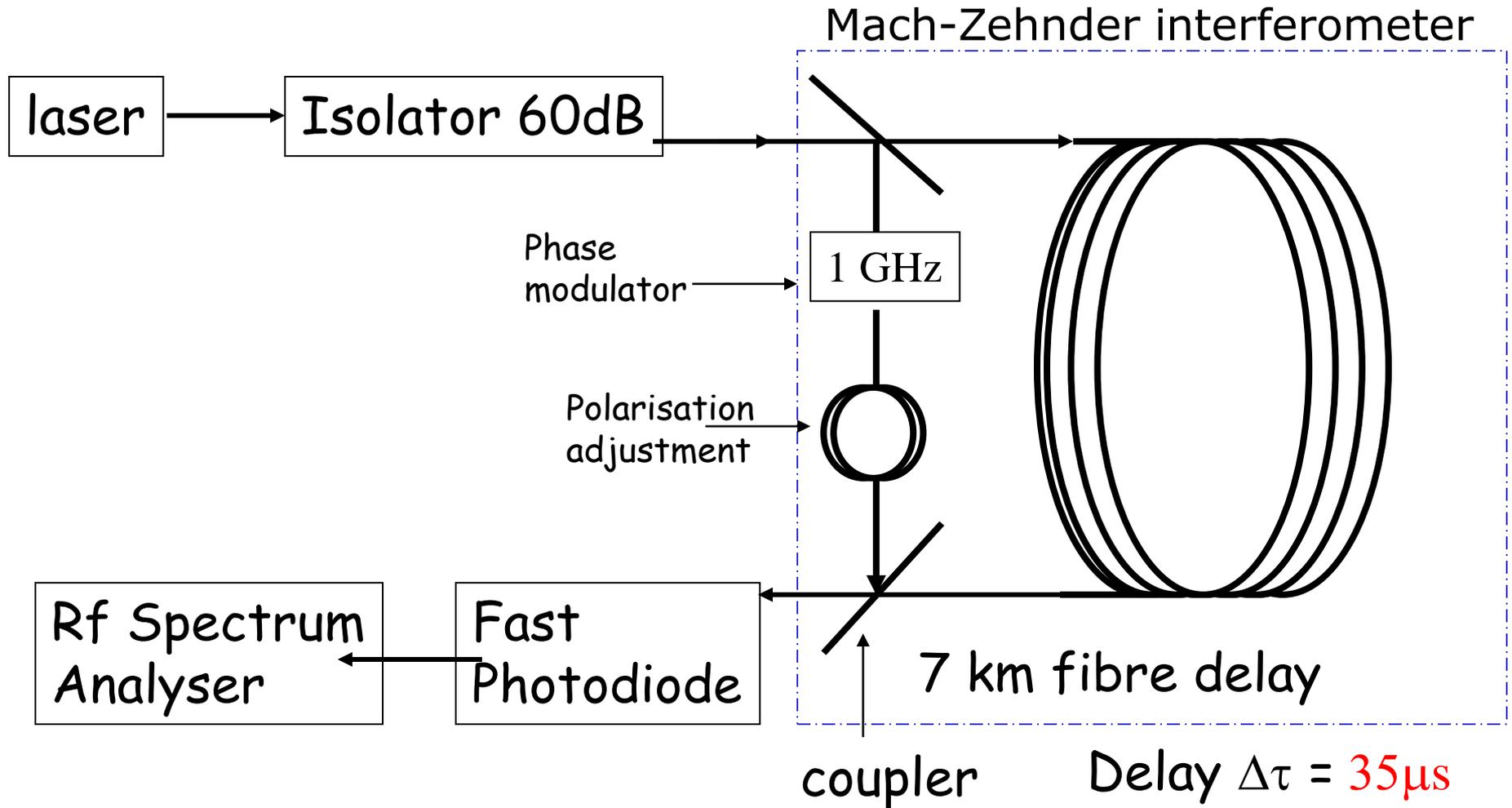
Incident light is split into 2 paths by the interferometer. One path is sent through a delay line (7km of fibre) if this delay is longer than the coherence length of the laser the 2 combining beams interfere as if they are from 2 independent lasers offset by the 1GHz.
