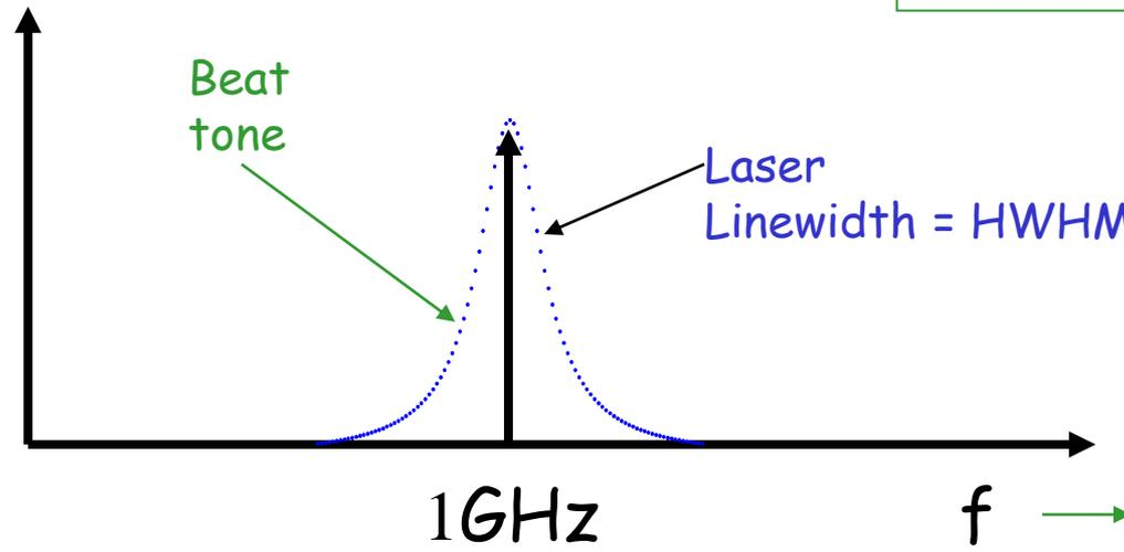
Delayed self-heterodyne measurement of DM laser with Lorentzian fit to extract linewidth
